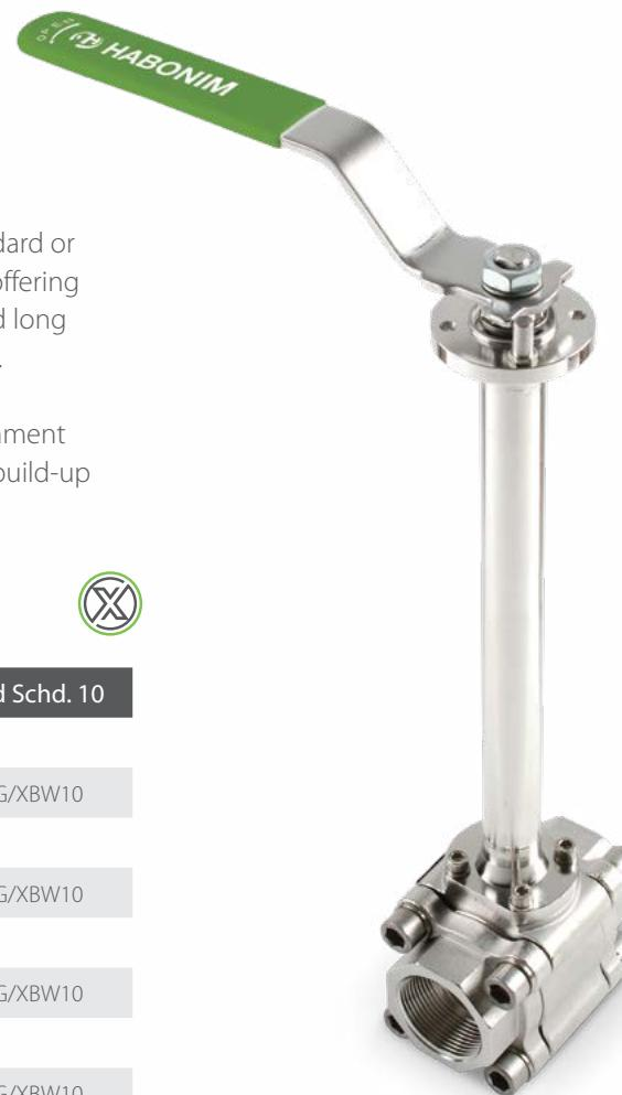
The C47 Series is Habonim Cryogenic 3-piece floating ball valve Standard or full port design equipped with the Total HermetiX Integrity Package offering tight shutoff, zero-emission, double body sealing, fire-safe design, and long service life with high durability. ANSI B16.34 Class 600 (wall thickness).
